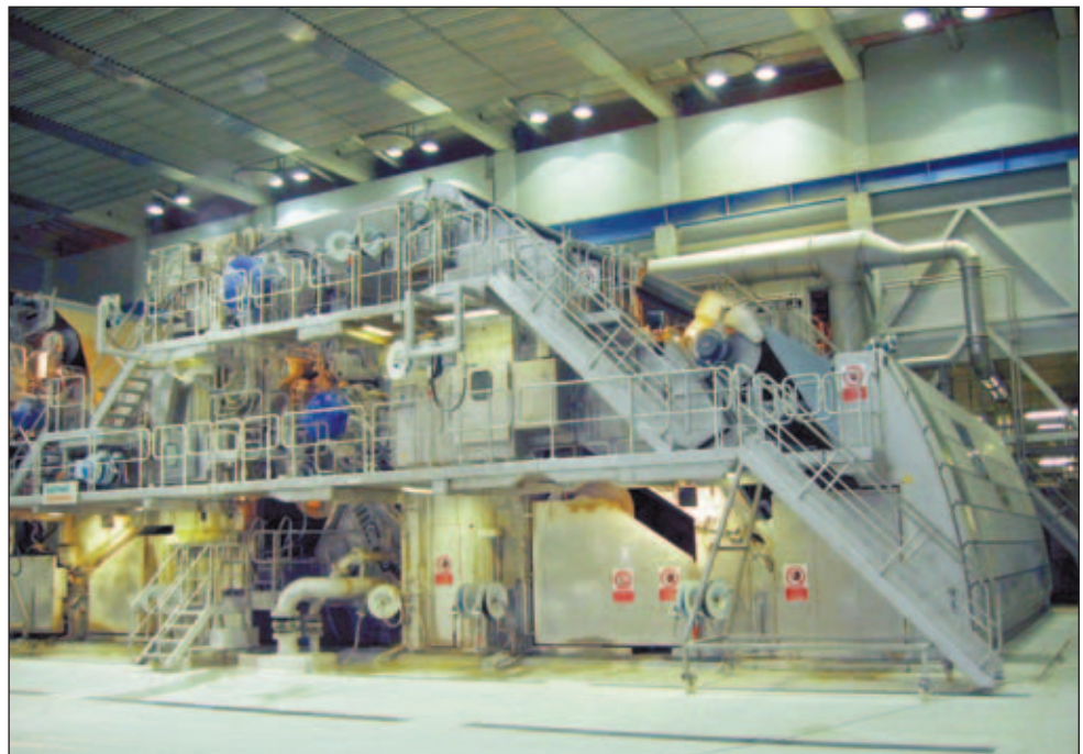
Figure 1 Verzuolo PM9, the flagship PM trims at 9.6m and produces 400,000 tpy of LWC grades in the 45 to 70 g/m 2 range
