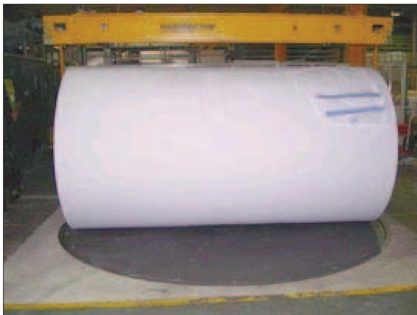
Georgia Pacific is using an air film turntable to streamline tissue reel handling at its South Wales mill and Sheffield plant.
