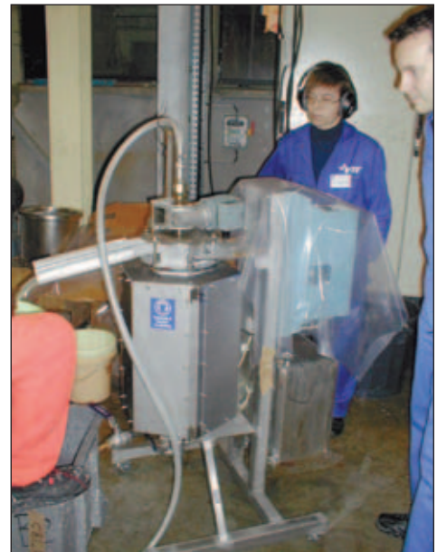
The ultrasound pilot device. Ultrasonic treatment is showing enormous potential for the de-inking of difficult inks. It will be covered next month, in Part 3 of this feature.
