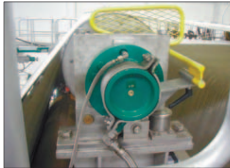
Figure 1: Press Felt Tension Measuring with bracket type load cell.
